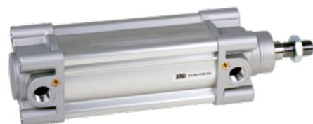
Double acting Al-profile cylinder with integrated sensor grooves, adjustable cushions and magnetic piston for proximity sensors. The sensors can be installed directly into the sensor grooves of the Al-profile. Standard stroke lengths in table below, additional lengths on request.
