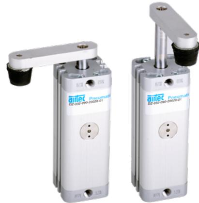
Double acting pneumatic cylinder with magnetic piston for proximity sensors and built-in cushioning rings. Due to the combination of linear and swivel movement of the piston rod, combined insertion and clamping operations can be realised. Special angles and special stroke lengths are available on request.
