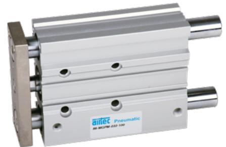
Double acting pneumatic cylinder with magnetic piston and built-in cushioning rings. The sensors can be installed directly into the sensor grooves of the Al-profile.
