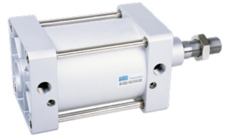
Double acting Al-profile cylinder with integrated sensor grooves, adjustable cushions and magnetic piston for proximity sensors. The sensors can be installed directly into the sensor grooves of the Al-profile.
