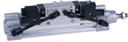
Double acting Al-profile cylinder with integrated sensor grooves, adjustable cushions and magnetic piston for proximity sensors. The sensors can be installed directly into the sensor grooves of the Al-profile. The cylinder includes a 5/2- or 5/3-way valve with a high flow rate and compact dimensions.
