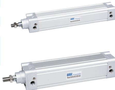
Double acting Al-profile cylinder with integrated sensor grooves, adjustable cushions and magnetic piston for proximity sensors. The sensors can be installed directly into the sensor grooves of the Al-profile. Standard stroke lengths in table below, additional lengths on request.
