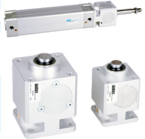
A BH rod lock with mechanical clamping is mounted on the front cylinder head. The rod lock is activated by spring force when at rest and is released by pressurisation.
