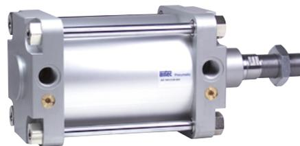
Double acting Al-profile cylinder with integrated sensor grooves, adjustable cushions and magnetic piston for proximity sensors. The sensors can be installed directly into the sensor grooves of the Al-profile.
